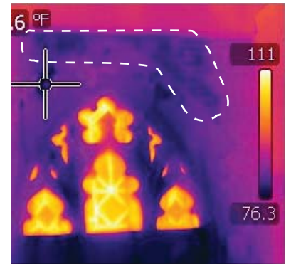
Infrared thermography shows trapped moisture in existing masonry.
